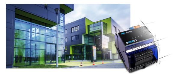
Microprocessor controlled digital counter module featuring 4 digital inputs. The serial line communication is based on Modbus RTU (RS485) protocol. Native modbus map grants seamless integration into variety of PLC/SCADA systems. Acquired values can be stored in the device temporarily as an extra protection against a short term power failure.
